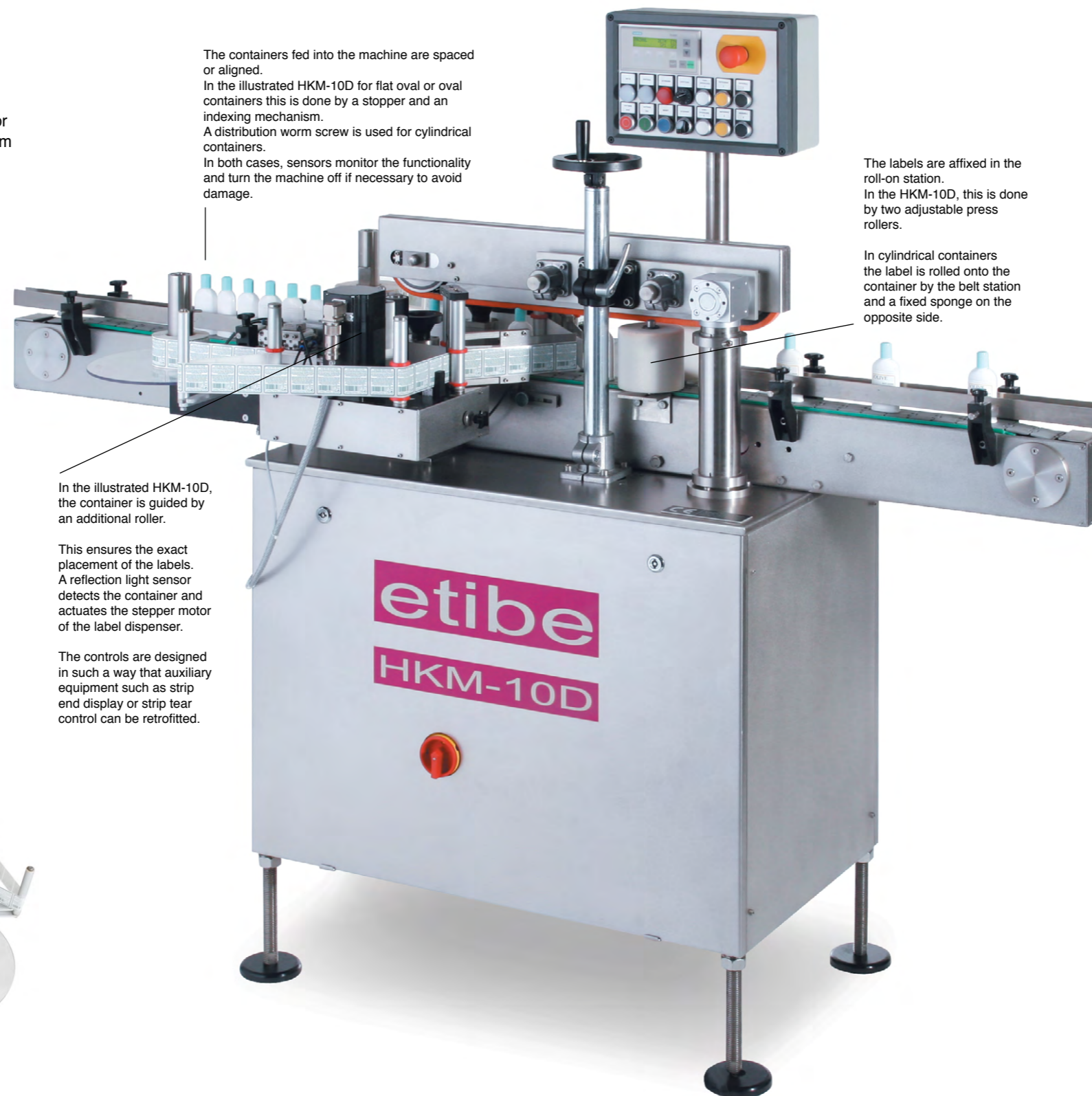
Model HKM-10D with a second label dispenser for back labels
